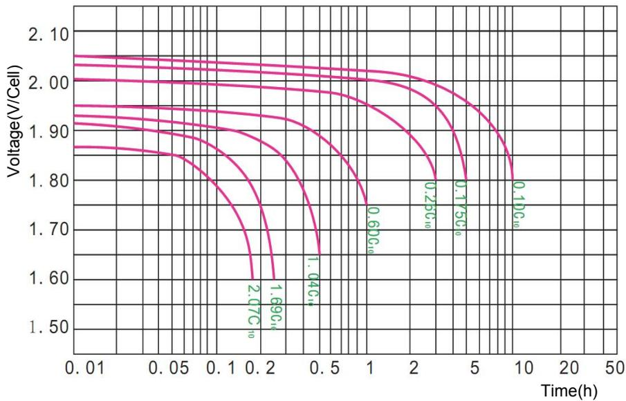
■ Table 2-1 GFMG series battery end voltage at different discharge rate(25 °C)
